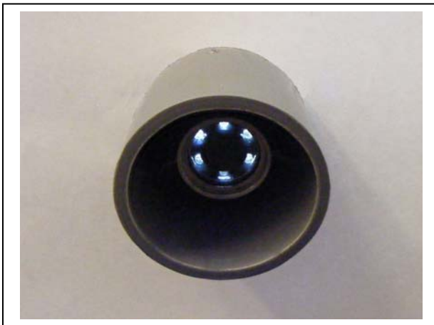
Lower end of tube showing illuminated camera
