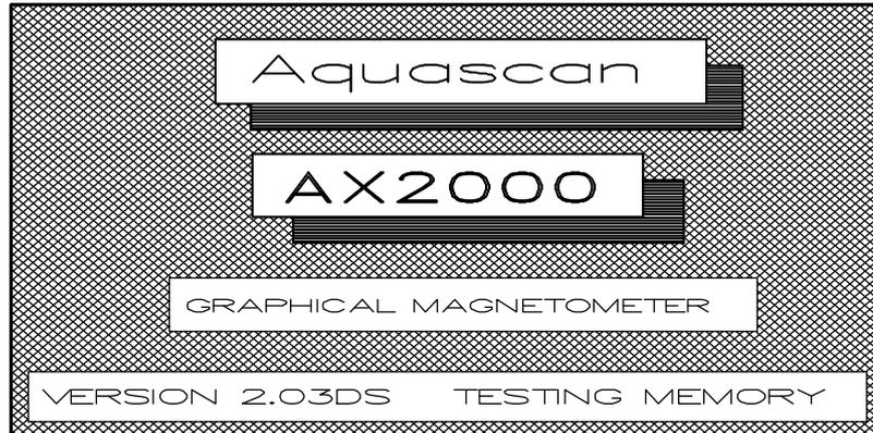
This screen will be present for approximately 10-15 sec's. During this time the AX2000 will perform its memory test. The words "TESTING MEMORY" will appear in the lower half of the screen and the sounder will emit a rapid burst of clicks. The version of software fitted to the AX2000 is also indicated. When the memory test has been successfully completed, a new screen will be display memory configuration installed e.g. 256Kbyte.
