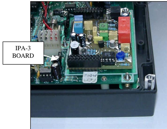
In order to change the area tuning zone of operation pre-tuned IPA-3 circuits are available and require to be substituted as follows.
