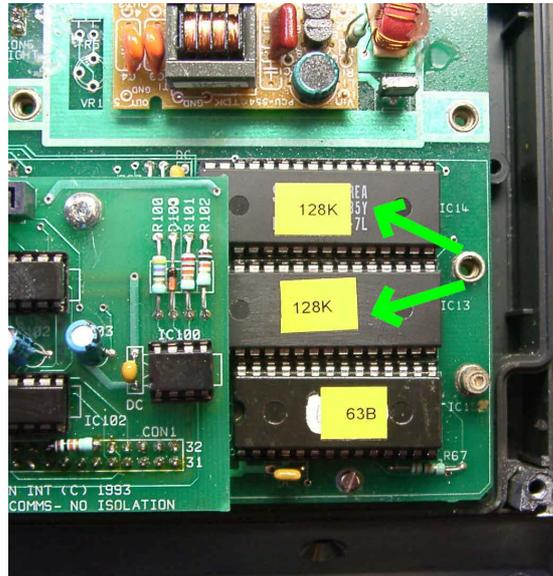
*The arrows above show the position of the RAM chips in an AX2000 PCB.*
