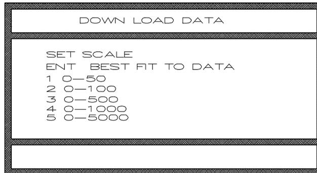
Pressing the ENT key instructs the AX2000 to automatically select the best-fit scale for the data to be printed on. The AX2000 achieves this by searching through the file to be printed, for the largest deviation. If possible, the scale selected will allow this maximum deviation to be printed.
