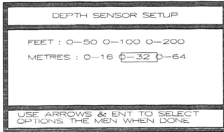
The above menu selection allows for the units displayed to be selected as feet or metres, this is effected by highlighting the required range in the relevant units and pressing the **ENT** key followed by the **MEN** key to return to the MAGNETOMETER MODE MENU.
