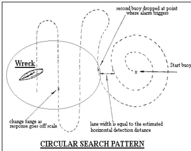
The circular search pattern is particularly suited when a graphical plotting navigator can be used in conjunction with the AX2000 magnetometer.
