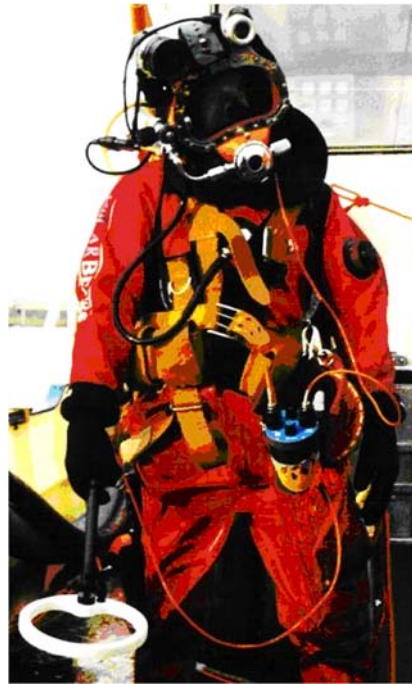
Diver prepared for EOD survey using AQ1B-Compact/20cm - Harness mounted
