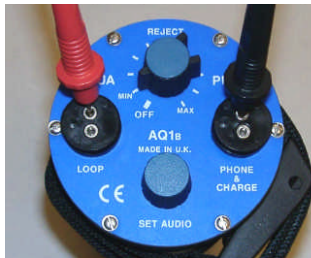
Battery Test Points
